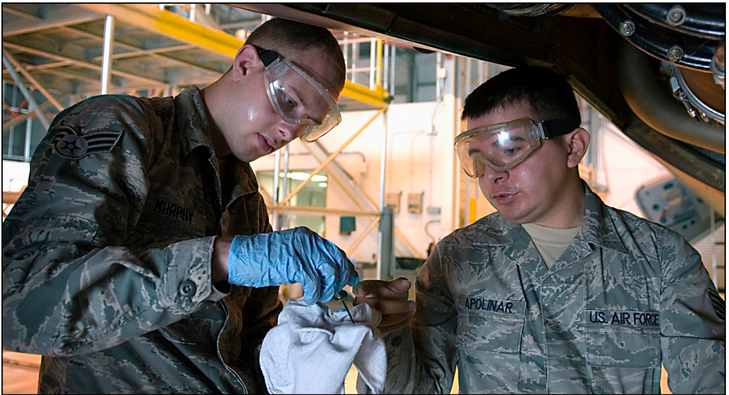
Senior Airman Daniel Apolinar, 434th Aircraft Maintenance Squadron aircraft electric and environmental system journeyman, trains Senior Airman Noah Murphy, 434th Aircraft Maintenance Squadron crew chief, on the proper procedures for changing air cycle machine oil on a KC-135R Stratotanker during a home-station check here at Grissom July 12.
