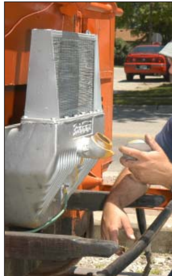
Sergeant McConnell checks the water level in the vaporizer. The vaporizer helps cool the 12-horse power single cylinder engine used on the railroad tracks.
