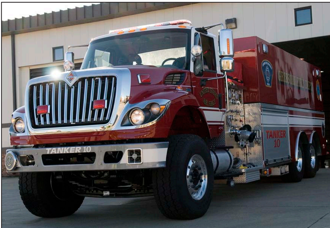
Grissom's new P26 tender tanker holds up to 4,000 gallons of water and is able to empty out 1,250 gallons of water per minute(U.S. Air Force photo/Senior Airman Damon Kasberg)
