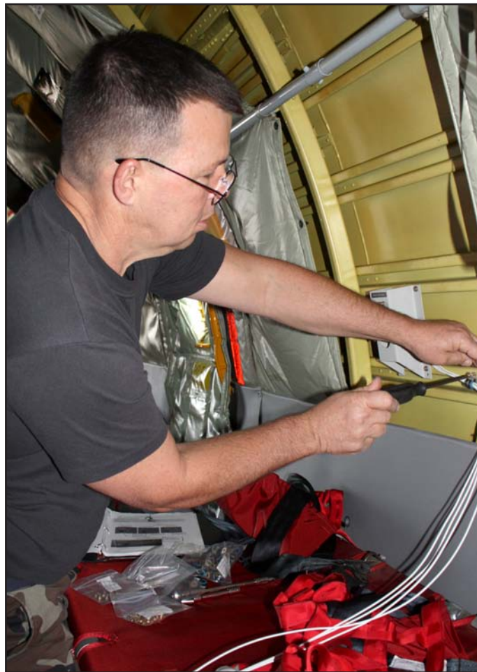
Photo by Staff Sgt. Ben Mota Master Sgt. Tom Patton, an electro environmental systems technician, installs outlets in a KC-135R stratotanker.
